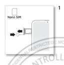
1 Insert the SIM tool into the tray hole to pop out the trav.
