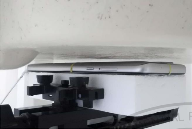
Back with handset, Test Separation 5 mm
