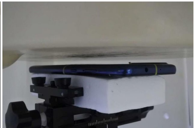
Back, Test Separation 9 mm
