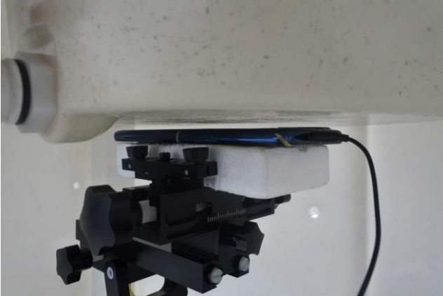
Back with handset, Test Separation 5 mm
