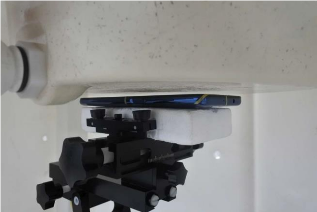
Front, Test Separation 5 mm
