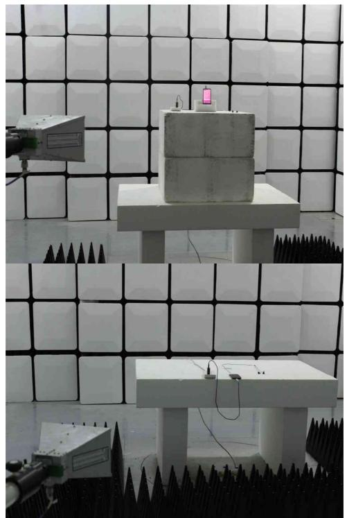
**1.3** Setup for Unwanted Emissions that fall Outside of the Restricted Bands(Radiated) and Unwanted Emissions in the Restricted Bands (Radiated) above 1GHz
