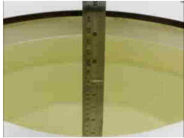
Fig 11.2 Photo of Liquid Height for Body SAR
