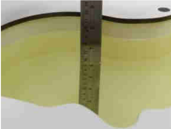
Fig 11.1 Photo of Liquid Height for Head SAR
