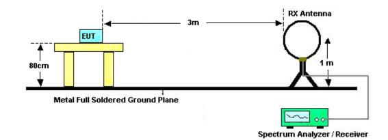
For radiated emissions from 30MHz to 1GHz
