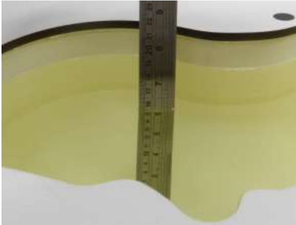
Fig 11.1 Photo of Liquid Height for Head SAR
