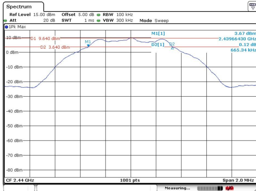
6 dB Bandwidth Plot on Channel 19
