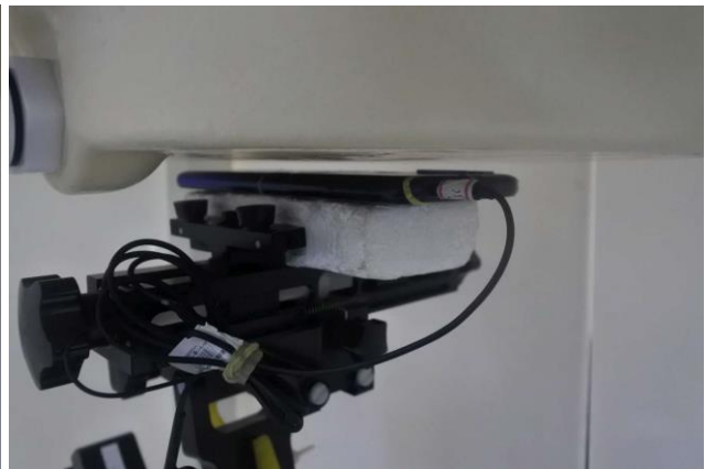
Back with handset, Test Separation 5 mm
