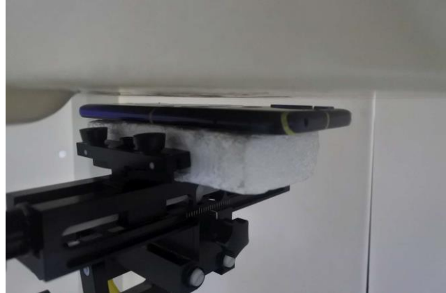
Back, Test Separation 5 mm
