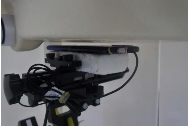
Back with handset 1, Test Separation 5 mm
