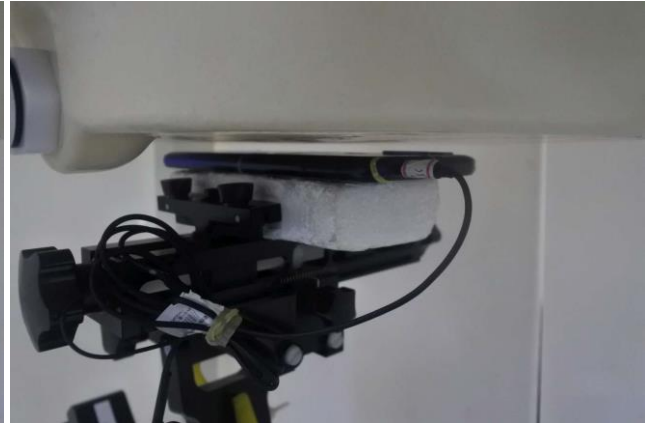
Back with handset 2, Test Separation 5 mm
