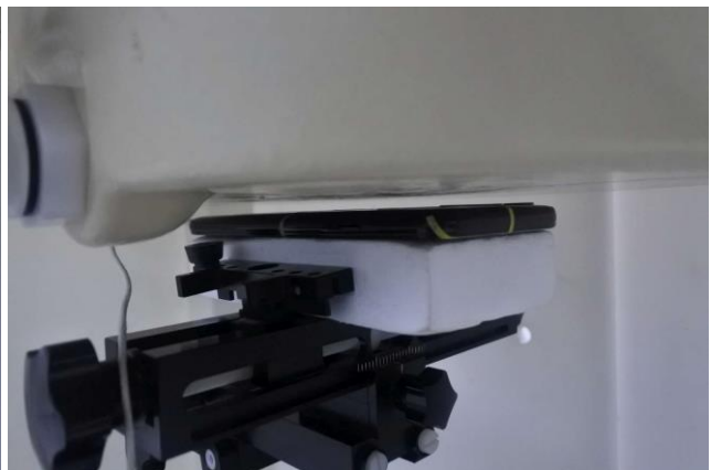
Back with headset, Test Separation 5 mm
