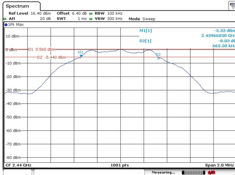
6 dB Bandwidth Plot on Channel 19
