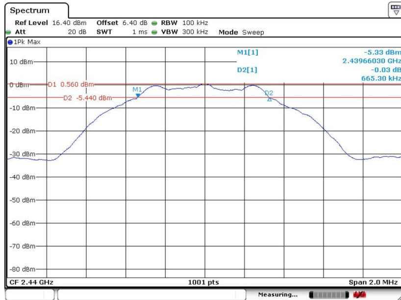
6 dB Bandwidth Plot on Channel 19
