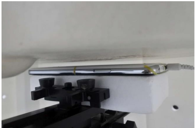
Back with handset, Test Separation 5 mm
