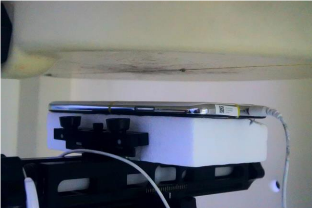
Back with handset, Test Separation 19 mm
