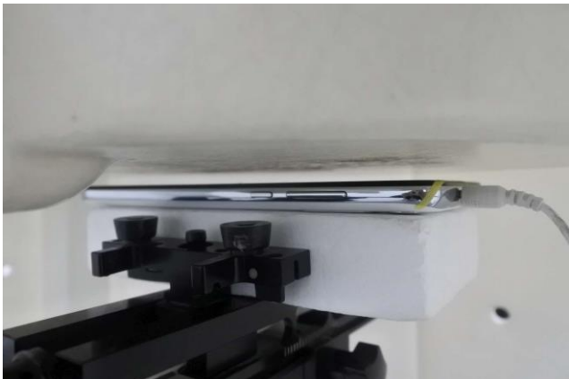
Front with handset, Test Separation 5 mm
