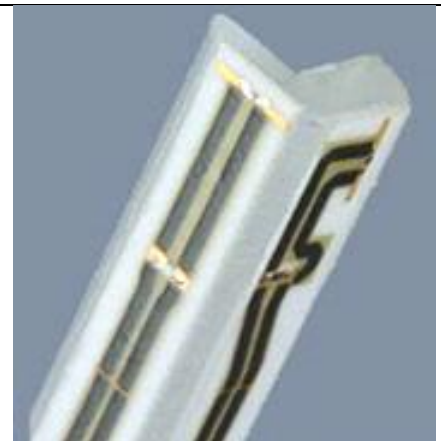
Fig 5.2 Photo of E-field Probe
