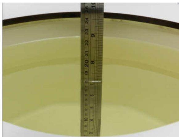
Fig 10.2 Photo of Liquid Height for Body SAR
