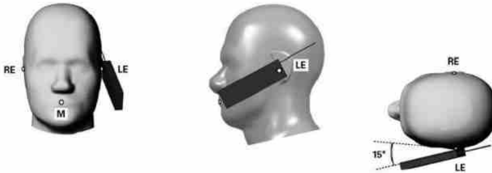
Fig 12.3.1 Tilt position. The reference points for the right ear (RE), left ear (LE), and mouth (M), which define the Reference Plane for handset positioning, are indicated.
