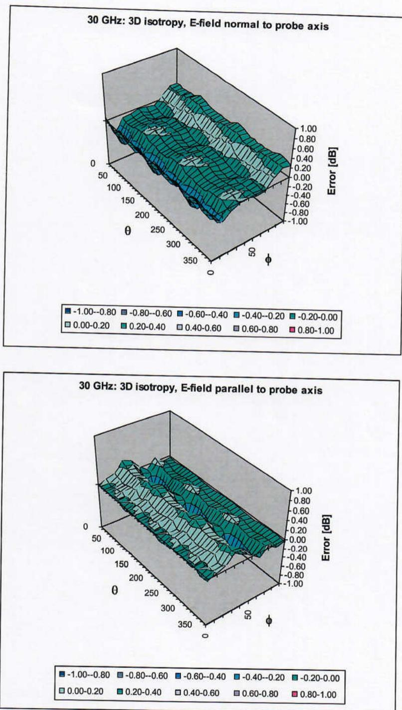
Probe isotropy for  $E_{\text{tot}}$ : probe rotated  $\phi = 0^\circ$  to  $360^\circ$ , tilted from field propagation direction  $\vec{k}$
