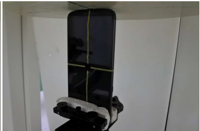
Bottom Side, Test Separation 0 mm
