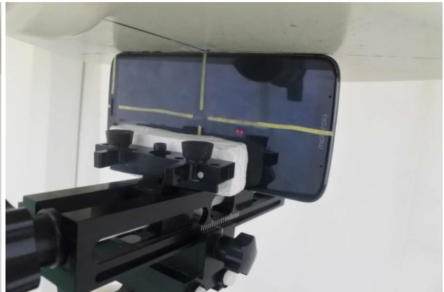
Right Side, Test Separation 0 mm
