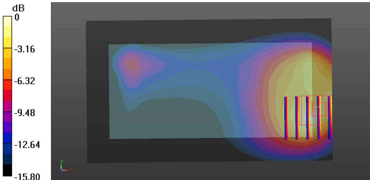
0 dB =  $2.87 \text{ W/kg}$  =  $4.58 \text{ dBW/kg}$
