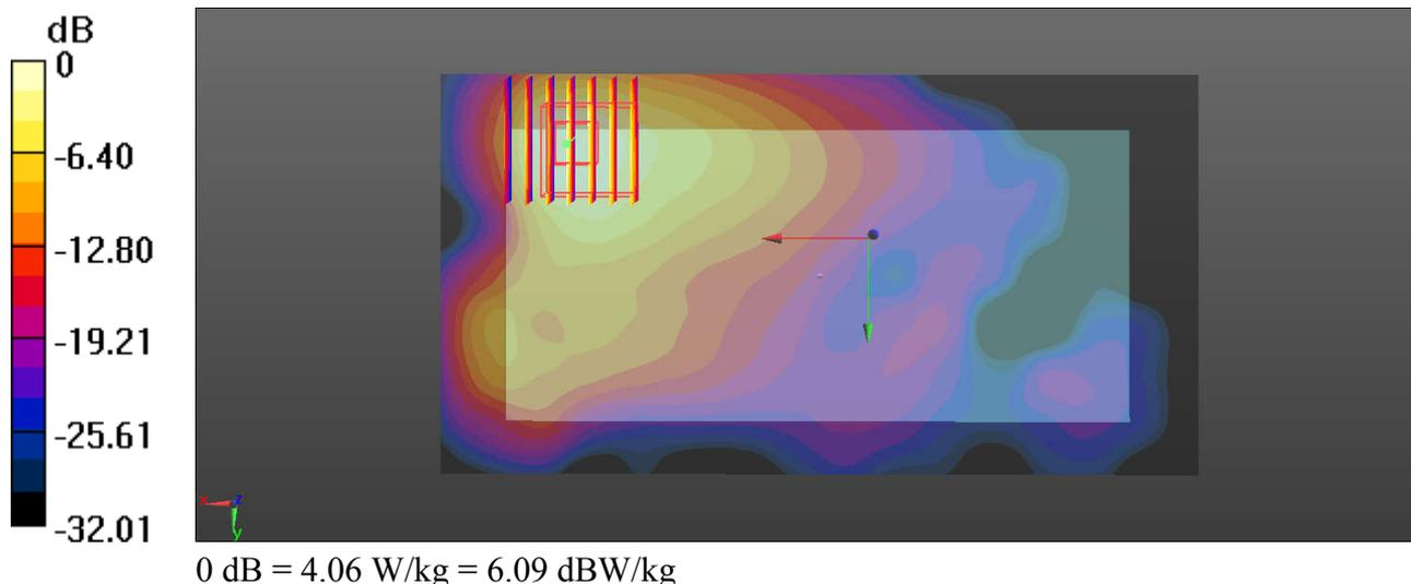
**59\_WLAN5GHz\_Band2 802.11a 6Mbps\_Left Side\_0mm\_Ant 1\_WPC\_Off\_Ch60**
