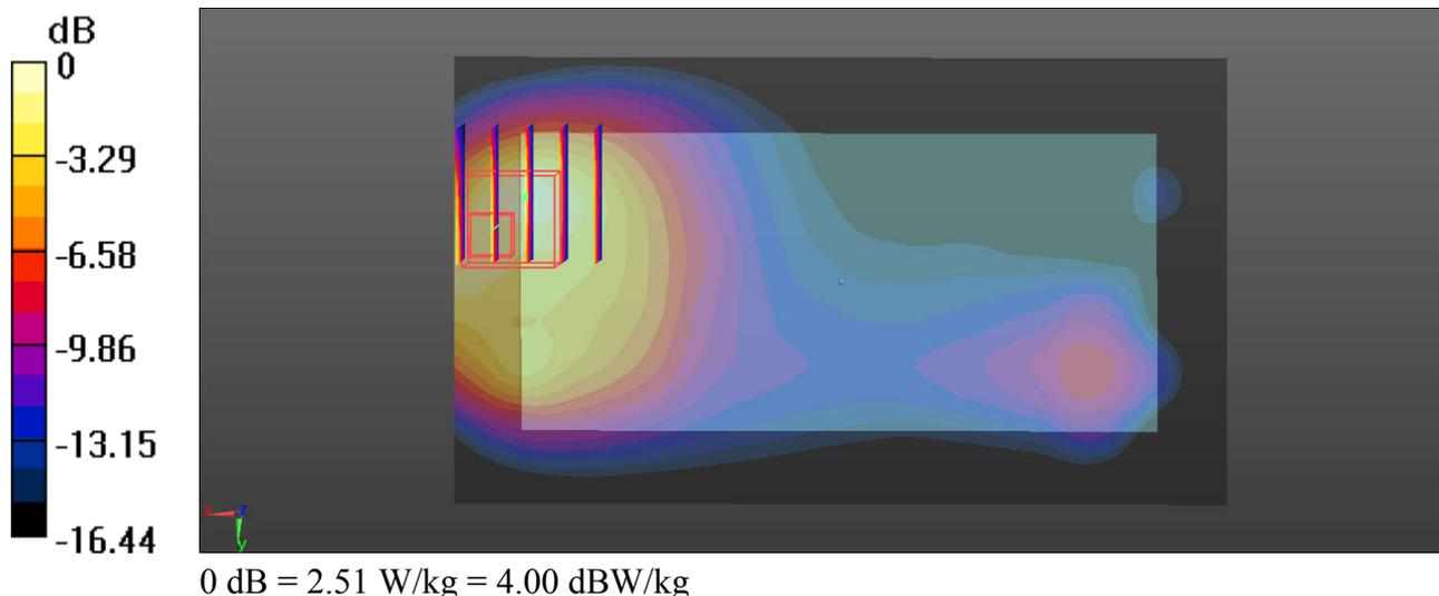
**56\_LTE Band 66\_20M\_QPSK\_50RB\_0Offset\_Back\_0mm\_WPC\_Extremity On\_Ch132072**
