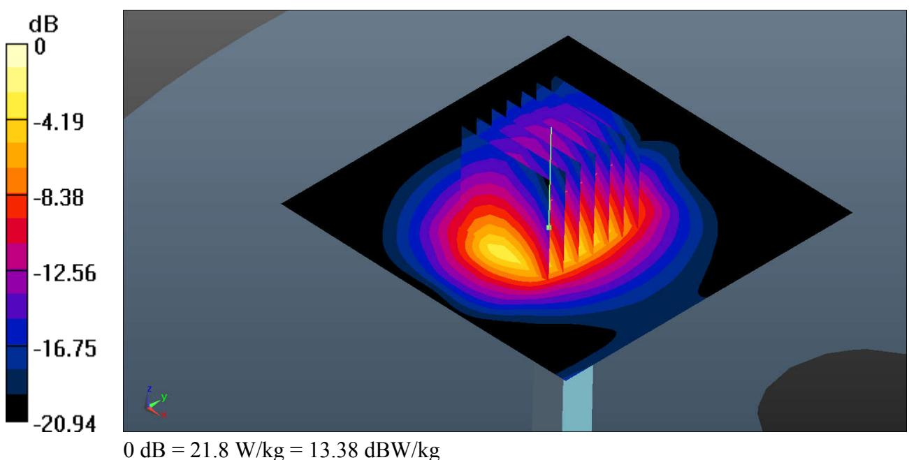
**System Check\_Body\_5250MHz****DUT: D5GHzV2-SN:1006**
