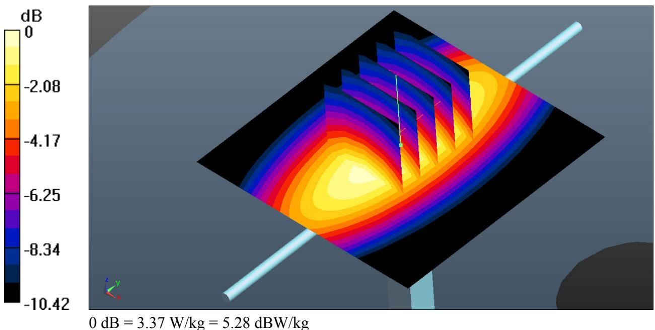
**System Check\_Body\_1750MHz****DUT: D1750V2 - SN:1069**
