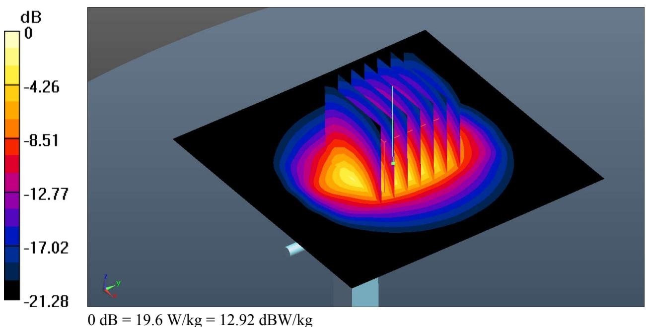
**System Check\_Body\_2600MHz****DUT: D2600V2 - SN:1061**
