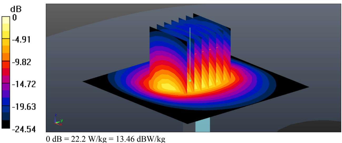
**System Check\_Head\_5250MHz****DUT: D5GHzV2-SN:1006**
