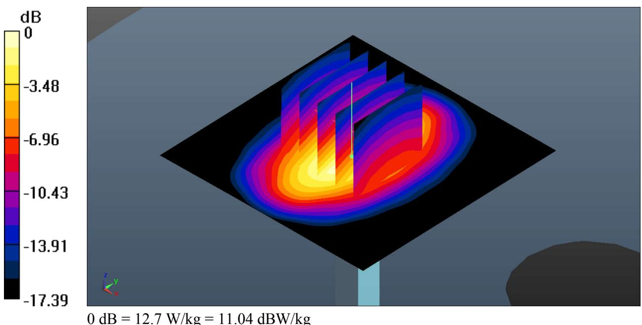
**System Check\_Head\_1900MHz****DUT: D1900V2 - SN:5d118**
