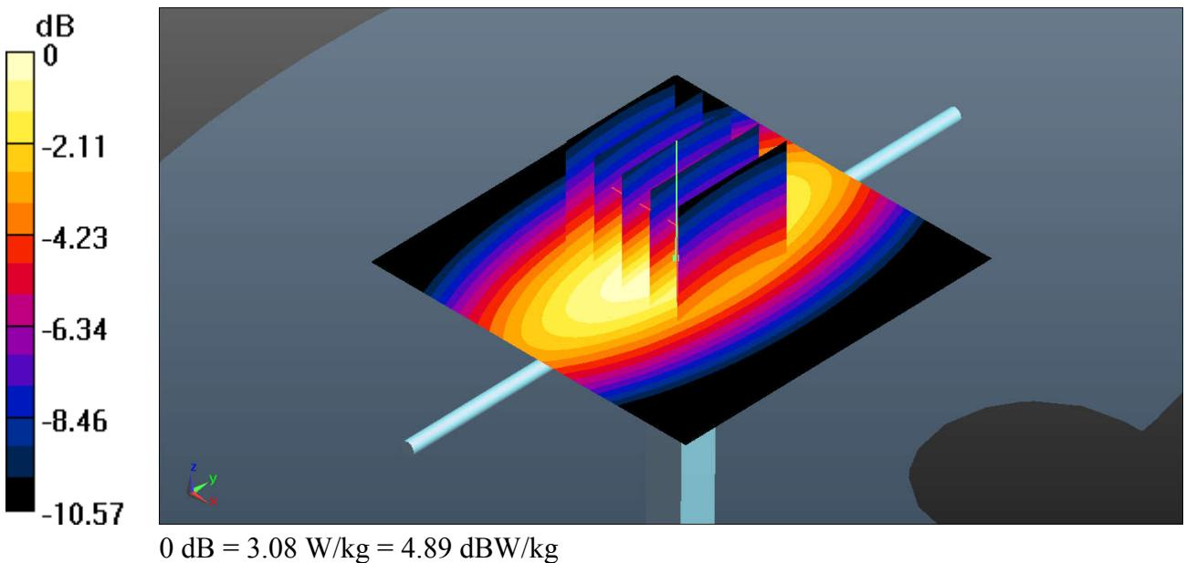
**System Check\_Head\_1750MHz****DUT: D1750V2 - SN:1069**
