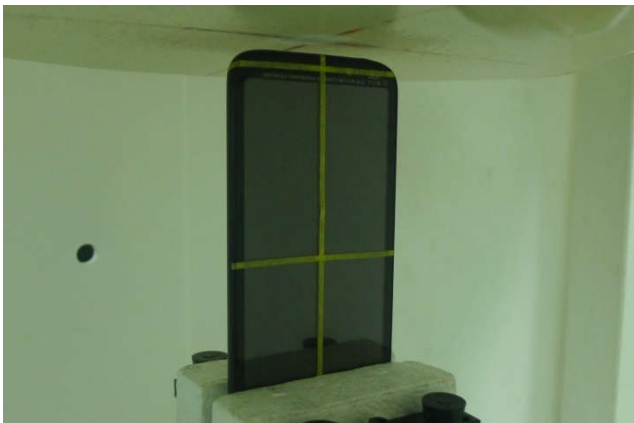
Top Side, Test Separation 5 mm
