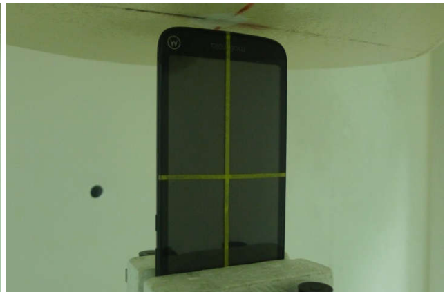
Bottom Side, Test Separation 5 mm
