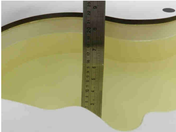
Fig 10.1 Photo of Liquid Height for Head SAR
