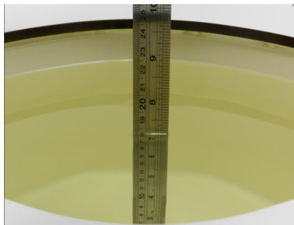
Fig 10.2 Photo of Liquid Height for Body SAR
