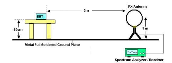
For radiated emissions from 30MHz to 1GHz
