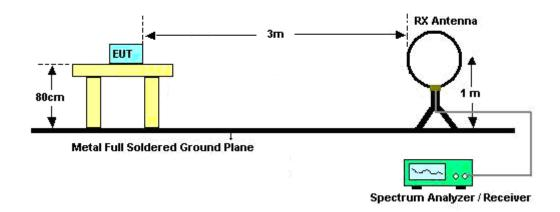
For radiated emissions from 30MHz to 1GHz
