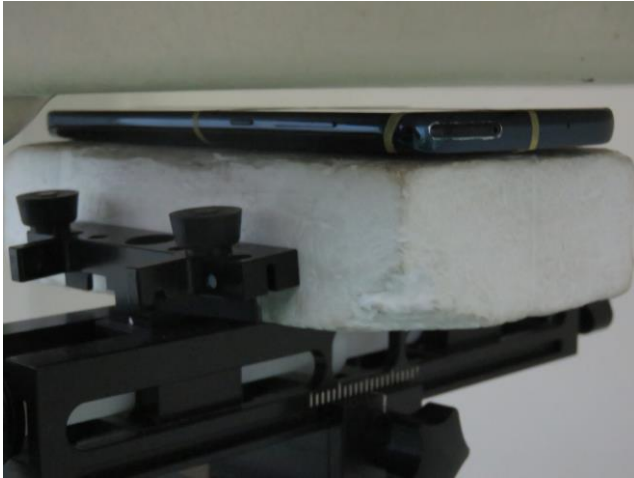
Front, Test Separation 5 mm
