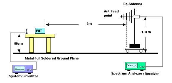
For radiated test above 1GHz
