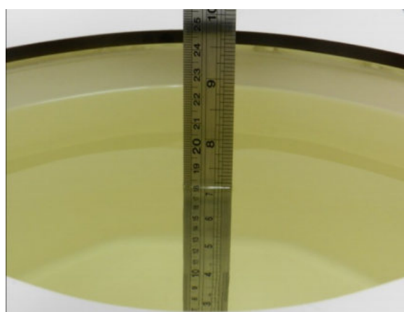
Fig 10.2 Photo of Liquid Height for Body SAR
