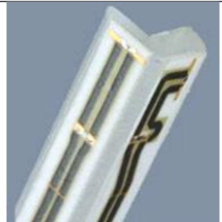
Fig 5.2 Photo of E-field Probe
