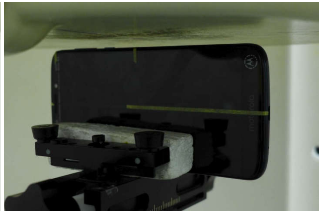
Right Side, Test Separation 5 mm
