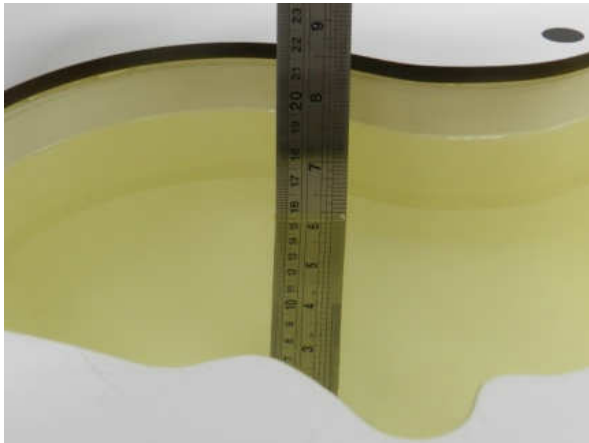
Fig 10.1 Photo of Liquid Height for Head SAR
