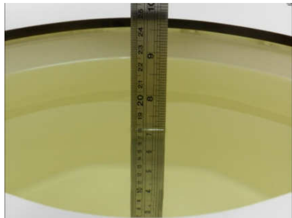
Fig 10.2 Photo of Liquid Height for Body SAR
