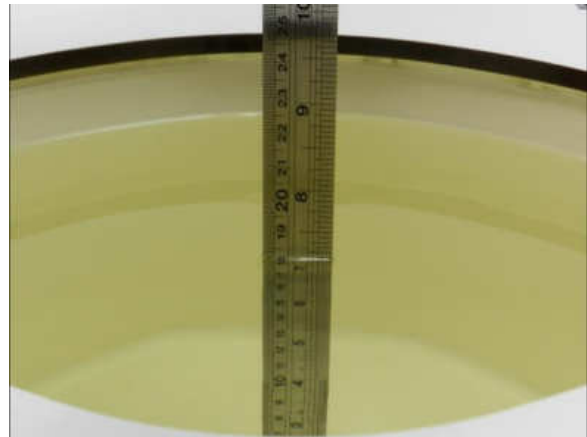
Fig 10.2 Photo of Liquid Height for Body SAR
