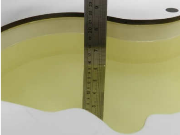
Fig 10.1 Photo of Liquid Height for Head SAR
