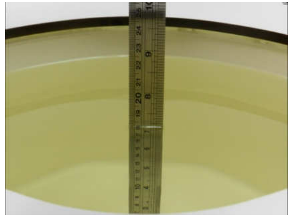
Fig 10.2 Photo of Liquid Height for Body SAR
