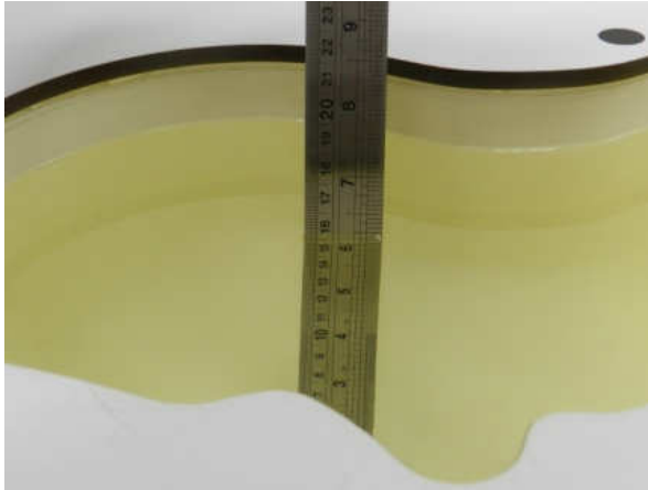
Fig 10.1 Photo of Liquid Height for Head SAR
