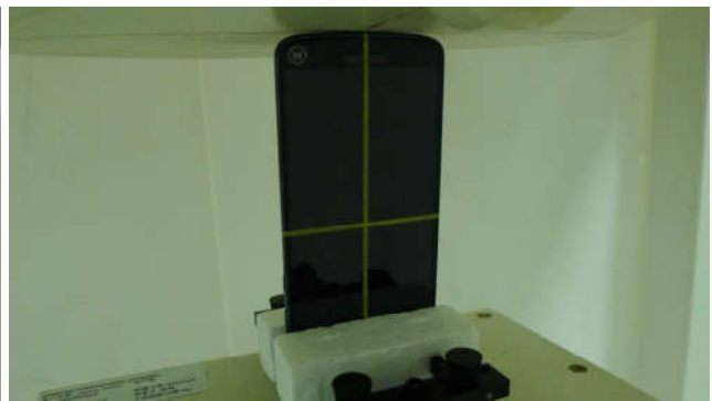
Bottom Side, Test Separation 0 mm
