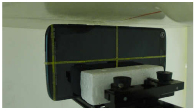
Right Side, Test Separation 5 mm
