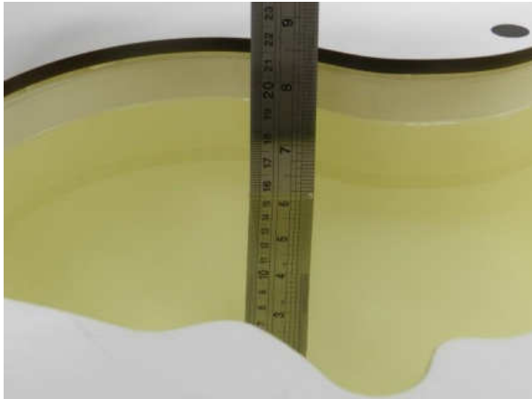
Fig 10.1 Photo of Liquid Height for Head SAR
