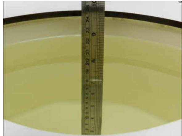
Fig 10.2 Photo of Liquid Height for Body SAR
