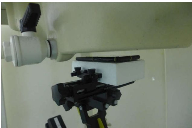
Front, Test Separation 10 mm
