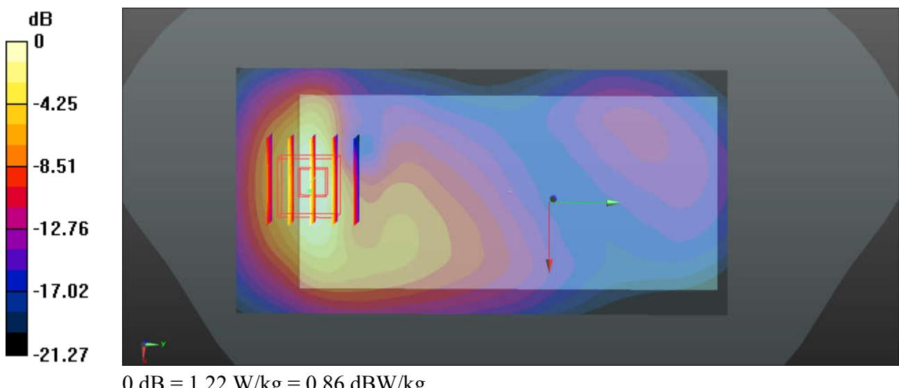
**36\_LTE Band 2\_20M\_QPSK\_1RB\_49Offset\_Back\_10mm\_\_Ch19100**
