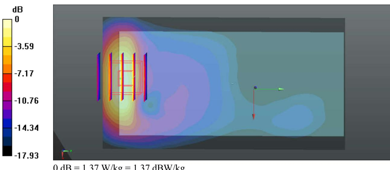
**37\_LTE Band 7\_20M\_QPSK\_1RB\_49Offset\_Back\_10mm\_21350**
