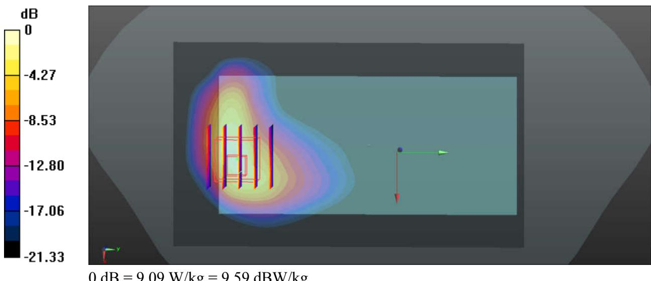
**46\_LTE Band 2\_20M\_QPSK\_50RB\_0Offset\_Back\_0mm\_Ch19100**
