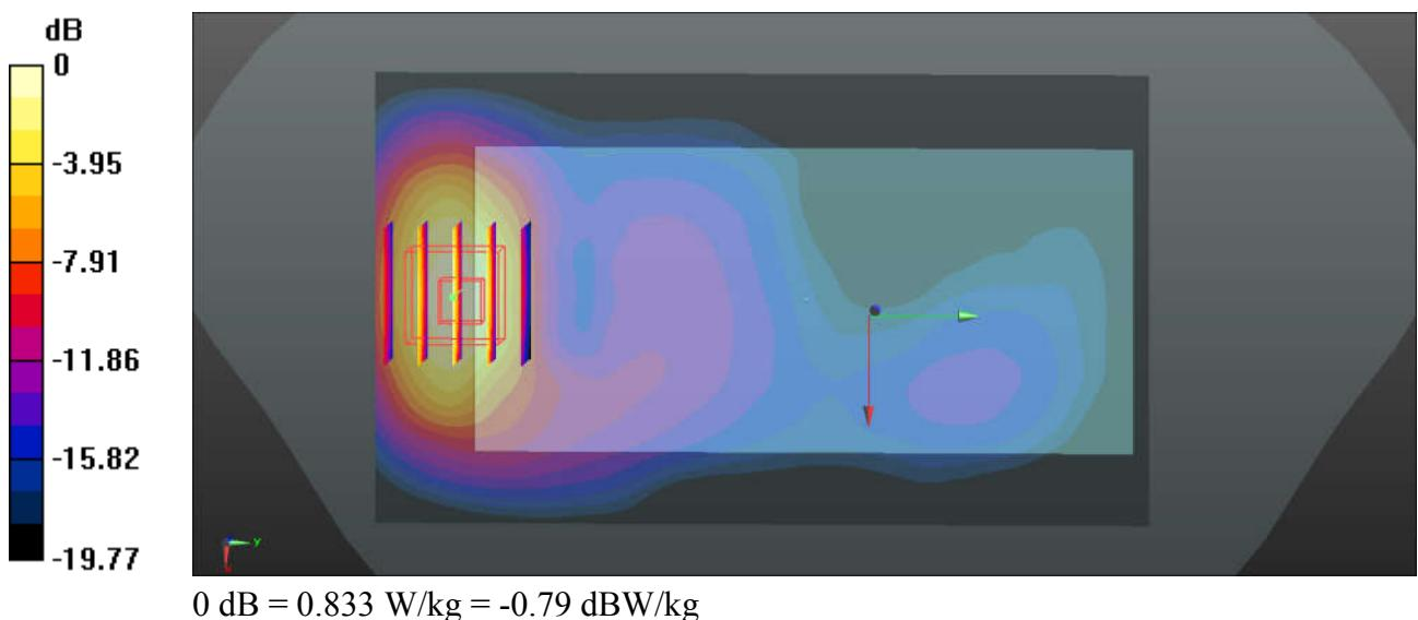
**33\_LTE Band 12\_10M\_QPSK\_1RB\_25Offset\_Back\_10mm\_Ch23095**
