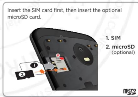
\* **Note:** To remove the SIM card, slide the lever on the slot.
