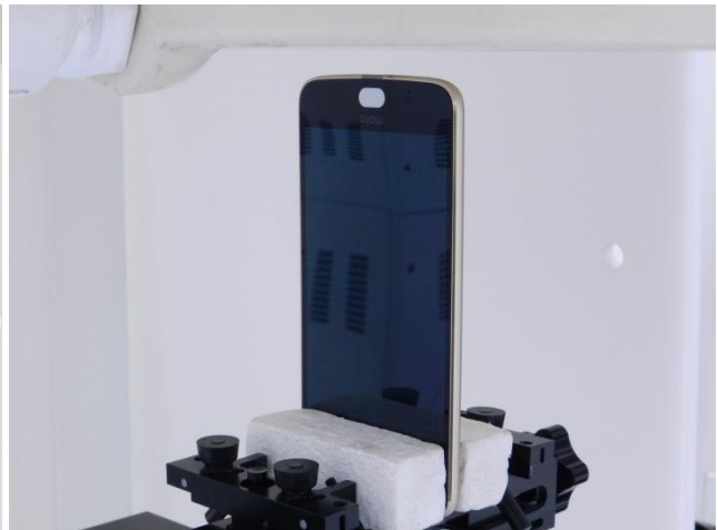
Bottom Side, Test Separation 10 mm
