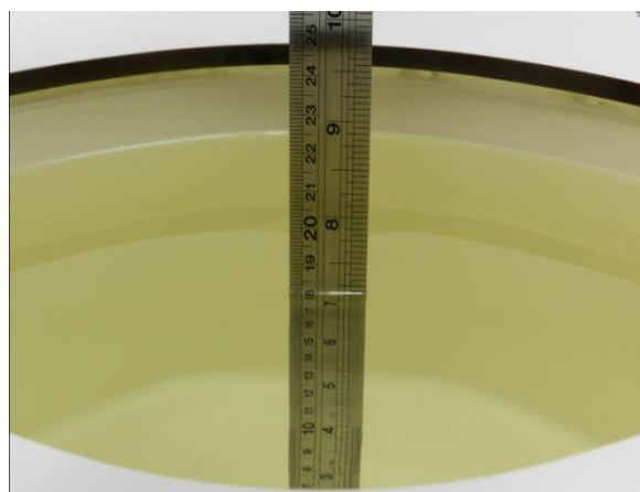
Fig 10.2 Photo of Liquid Height for Body SAR
