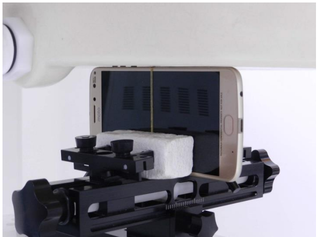
Right Side, Test Separation 0 mm
