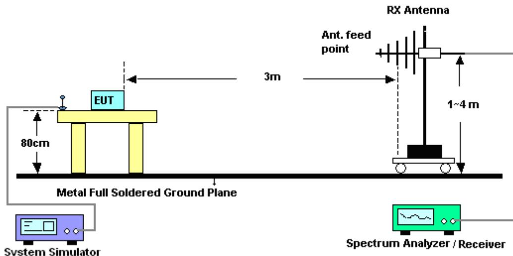
For radiated test above 1GHz
