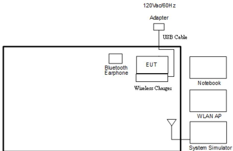
**<AC Conducted Emission with PMA Charging Mode>**
