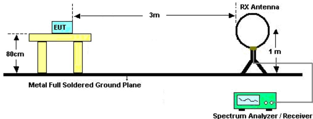
For radiated emissions from 30MHz to 1GHz
