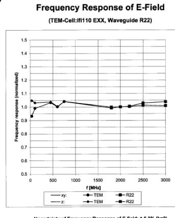
Figure 5-2 E-Field Probe Frequency Response
