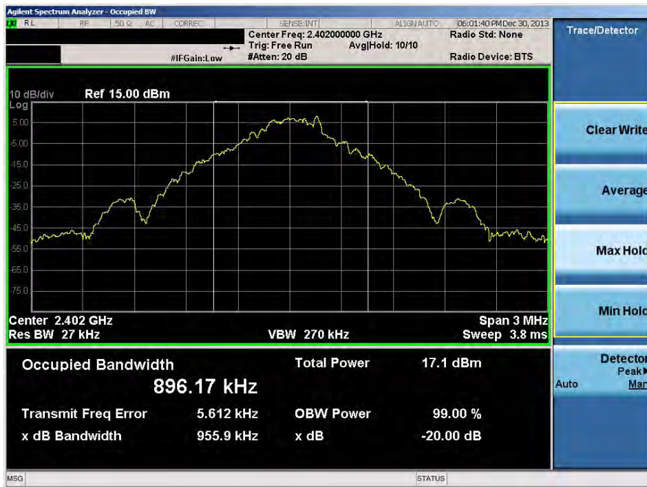
Plot 6-1. 20dB Bandwidth Plot (Bluetooth, 1Mbps – Ch. 0)
