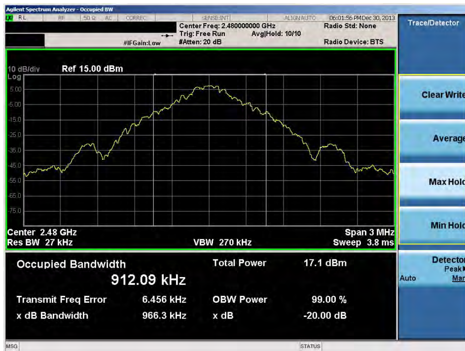
Plot 6-3. 20dB Bandwidth Plot (Bluetooth, 1Mbps – Ch. 78)
