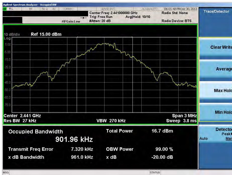
Plot 6-2. 20dB Bandwidth Plot (Bluetooth, 1Mbps – Ch. 39)
