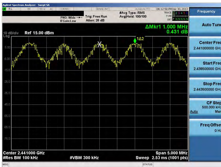
Plot 6-32. Channel Spacing Plot (Bluetooth)
