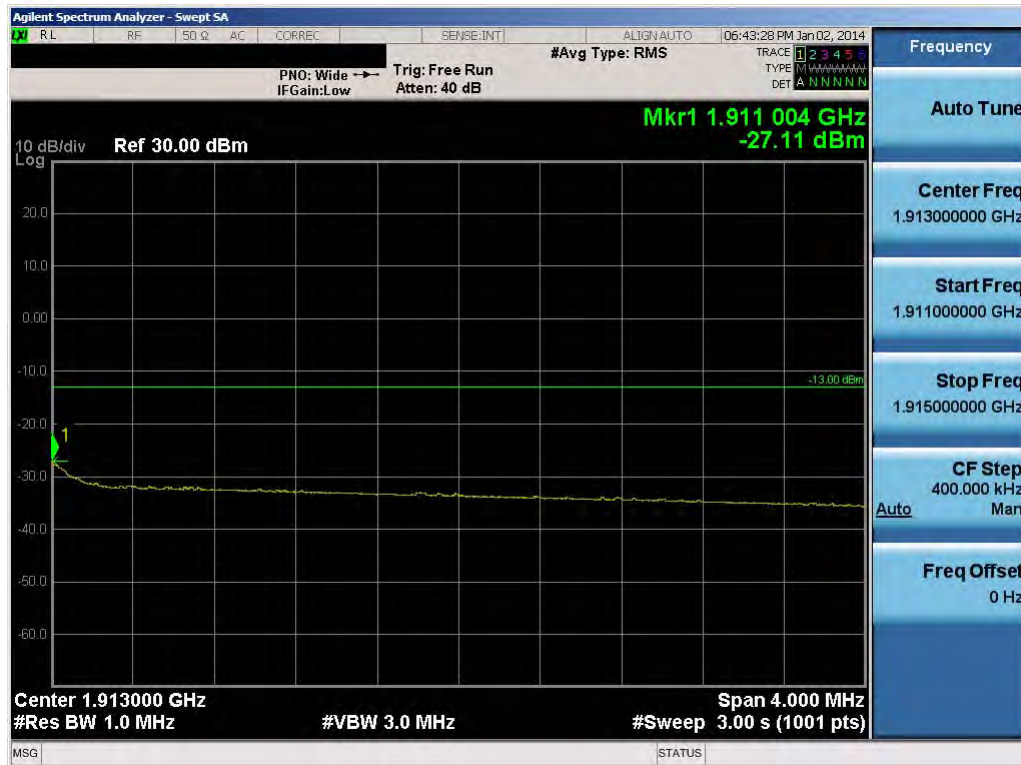
Plot 10-54. Upper Extended Band Edge Plot (10.0MHz QPSK – RB Size 50)
