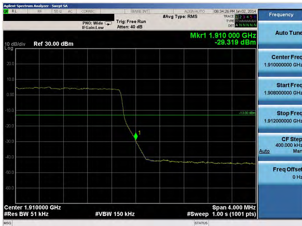
Plot 10-39. Upper Band Edge Plot (5.0MHz QPSK – RB Size 25)
