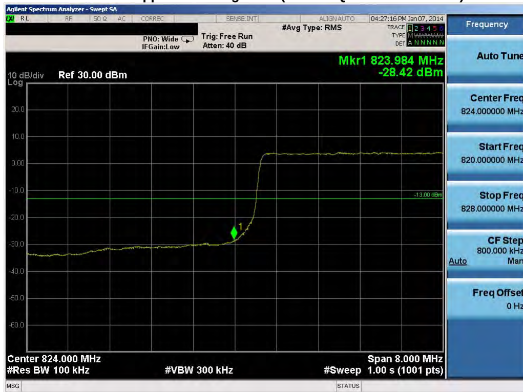
Plot 8-31. Lower Band Edge Plot (10.0MHz QPSK - RB Size 50)
