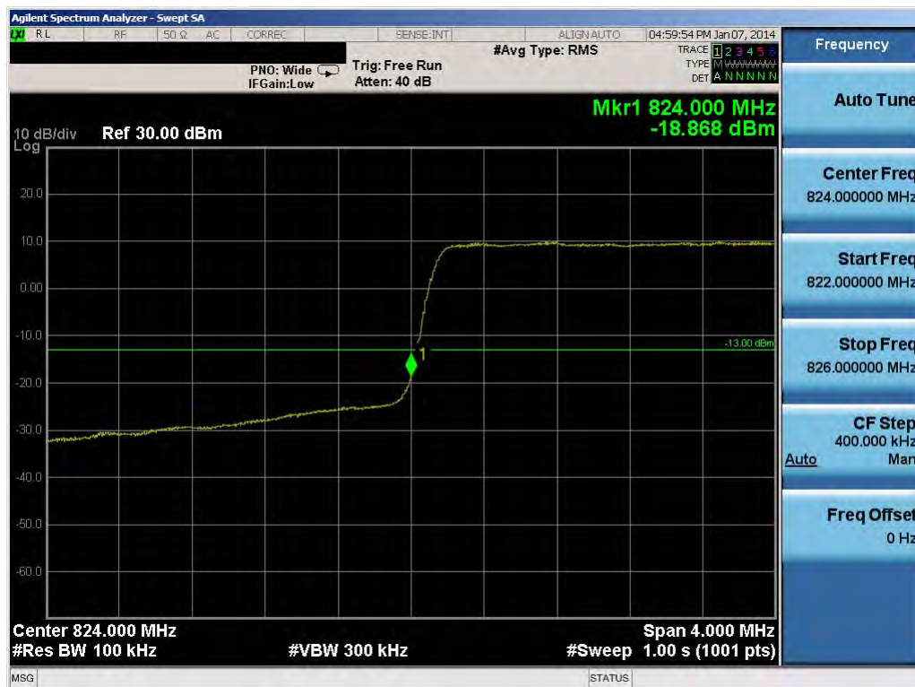
Plot 8-11. Lower Band Edge Plot (3.0MHz QPSK – RB Size 15)
