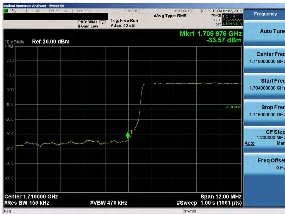
Plot 9-57. Lower Band Edge Plot (15.0MHz QPSK – RB Size 75)
