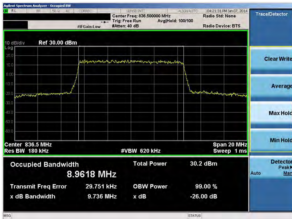
Plot 8-33. Occupied Bandwidth Plot (10.0MHz 16-QAM – RB Size 50)
