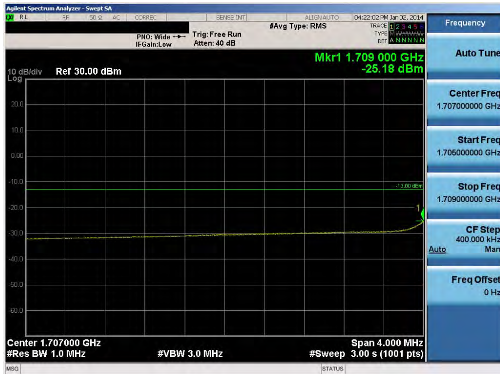
Plot 9-44. Lower Extended Band Edge Plot (10.0MHz QPSK – RB Size 50)
