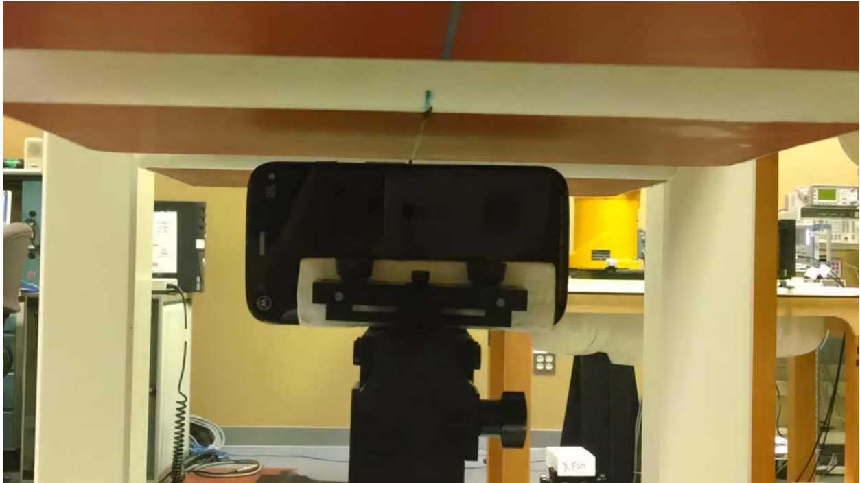
Figure 8: Mobile Hotspot Position, Long Edge of Phone facing Phantom (10 mm separation)
